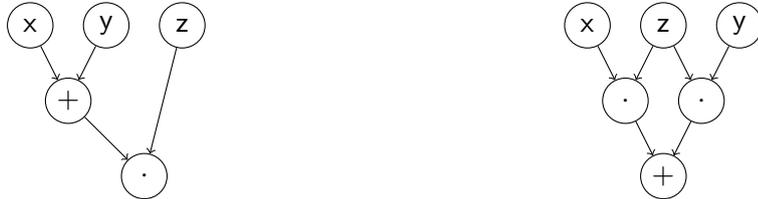
Figure 5.1: The picture shows two straight-line programs for evaluating the polynomial  $f(x, y, z) = (x + y)z$ . Let  $I = ([-1, 0], [1, 1], [0, 1])^T$ . Then, the program on the left evaluated at  $I$  yields  $f(I) = ([-1, 0] + [1, 1])[0, 1] = [0, 1]$ , while the program on the right yields  $f(I) = [-1, 0][0, 1] + [1, 1][0, 1] = [-1, 1]$ .
